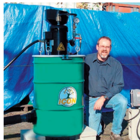
Mark Vinchoff, designer, displays the iCON concentrator that has been built for the small-scale alluvial miner. Photos by Ellsworth Dickson.
