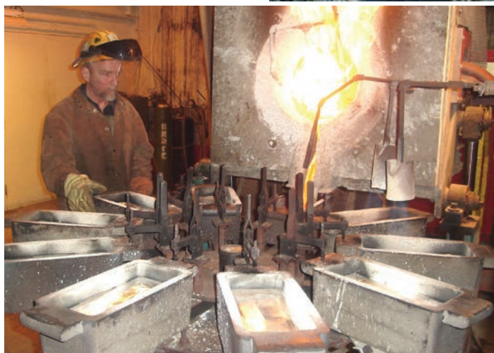
A worker pours 1,000-ounce silver bullion bars at Formation Capital's Sunshine Precious Metals Refinery in the Coeur d'Alene Mining District, northern Idaho. Photo courtesy Formation Capital Corp.
